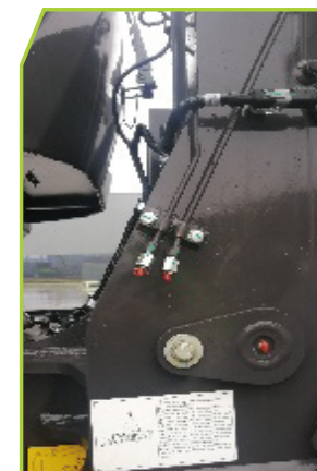
Grease lubrication points are centrally led out for ground-level access, enabling convenient daily maintenance.
