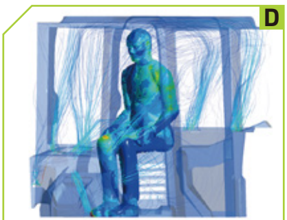
The cab is hermetically sealed with a pressure of +50 Pa, and equipped with N95-class filter elements, with a PM2.5 filtration efficiency of \geq 99\%
