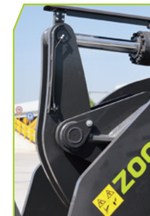
Grease lubrication points are centrally led out for ground-level access, enabling convenient daily maintenance.
