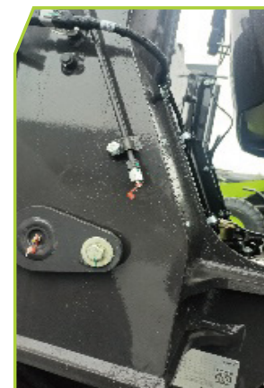
Grease lubrication points are centrally led out for ground-level access, enabling convenient daily maintenance.
